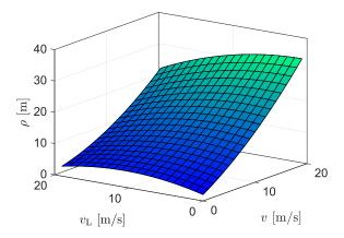
Fig. 9. Value of the function  $\rho$  defined in (49), which defines the minimum safe following distance as a function of the leader's velocity  $v_{\rm L}$  and truck velocity v.
