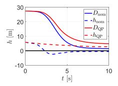
Fig. 12. (Left) Example profile for acceleration  $a_L$  of lead vehicle used in numerical simulation. (Center) Velocity  $v_L$  of lead vehicle (black) and velocity of the truck using the nominal controller (53) (blue) and safety-critical controller (57) (red). (Right) Following distance D and value of CBF h using the nominal controller and safety-critical controller.
