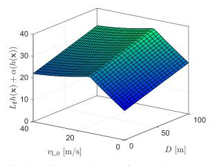
Fig. 10. Value of  $L_t h(\mathbf{x}) + \alpha(h(\mathbf{x}))$  as defined in (52) when  $L_g h(\mathbf{x}) = 0$  for various distances. As the function is strictly positive over the domain of interest, h is a CBF on  $\mathcal{C}$  for (46).
