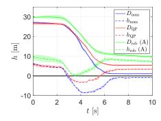
Fig. 15. (Left) Following distance and value of ISSf-CBF using the nominal controller (blue), safety-critical controller (red), and robust safety-critical controller (green) in the disturbed simulation. (Right) Mean value (lines) and standard deviations (fills) of the distance *D* and the ISSf-CBF *h* using the nominal controller (blue), safety-critical controller (red), and robust safety-critical controller (green) in experiment.
