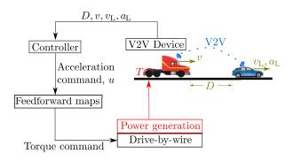
Fig. 8. Connected automated truck following a connected vehicle.
