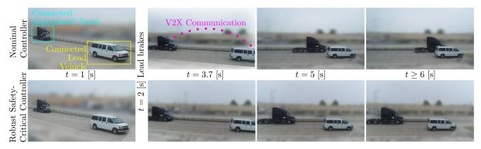
Fig. 1. Experimental configuration for heavy-duty CAV problem. (Top) Controller design without robustifying element yields safety violation. (Bottom) Robust safety-critical controller ensures CAV brakes early and aggressively enough to maintain safe distance.
