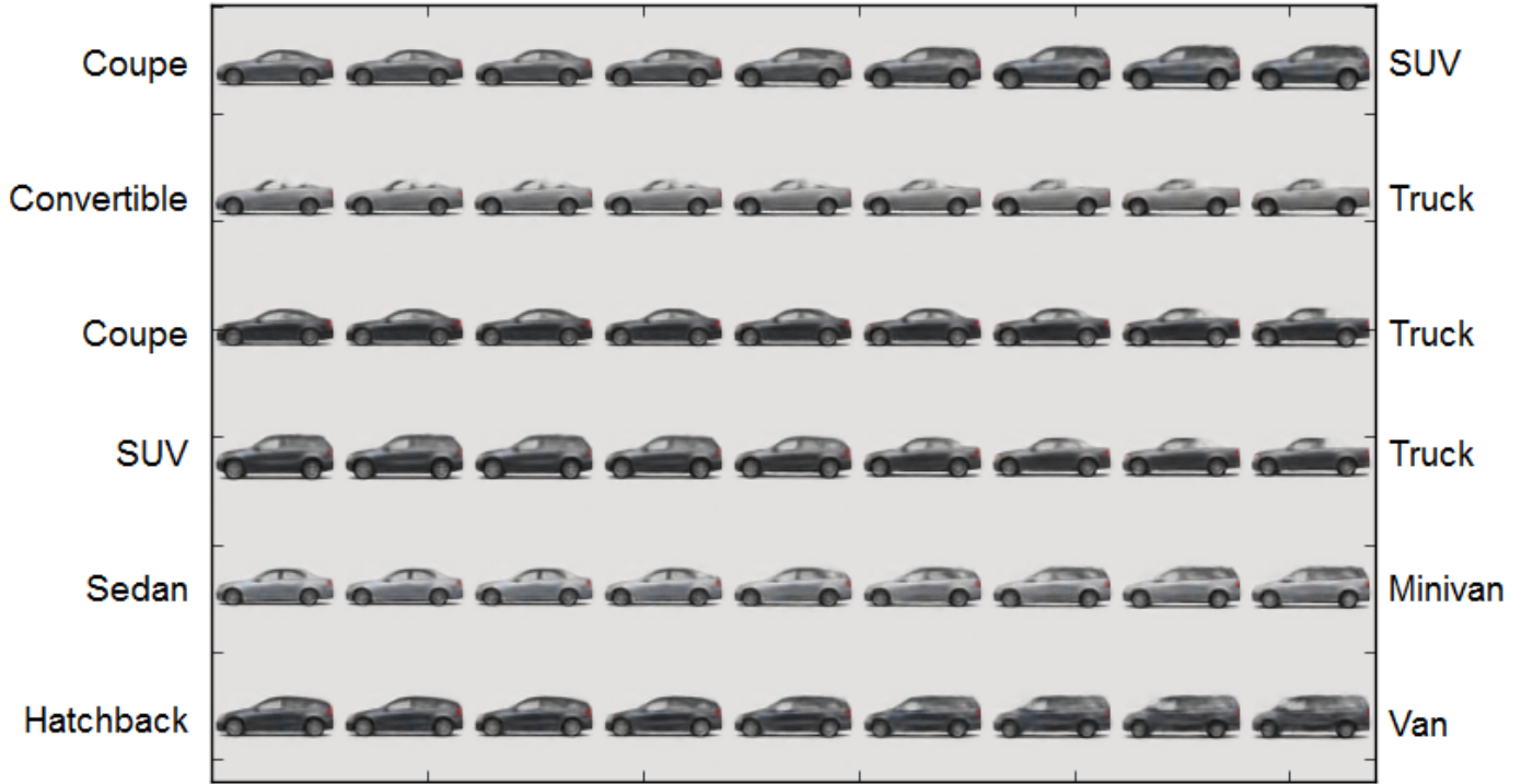
FIGURE 4. MORPHING BETWEEN VARIOUS BODY TYPES FROM THE ESTIMATED PRODUCT FORM DESIGN SPACE.
