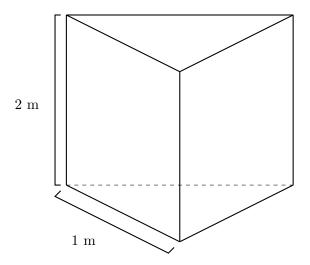
Solution: We take a horizontal slice at height y meters from the bottom of the tank. It has mass  $1325 \cdot \frac{\sqrt{3}}{4} 1^2 \Delta y$ . We need to move it 2 - y meters up. Thus, the work needed to pump all the chocolate to the top is
