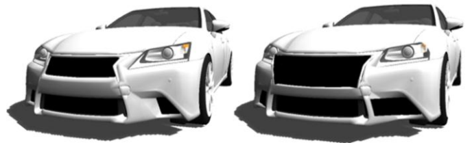
Figure 4: Example baseline 3D model and customer-morphed 3D model used during the 3D representation and design portion of the experiment. These models are morphable so that customers are able create conceptual designs to achieve a given design attribute using the crowdsourced web application. Similar to the 2D representation, these 3D models did not contain brand logos
