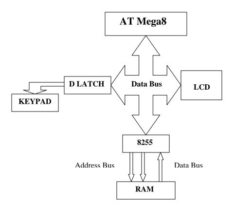
The **32kx8 bit RAM** has 28 pins, 15 address pins and 8 I/O pins. In addition to this there are 3 control signals. One to select the chip and the other two are to enable the chip in read or write mode. Keeping in mind the heavy requirement of port pins by the memory, an 8255 was introduced, to extend our ports.
