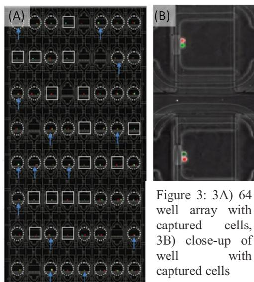
Figure 3: 3A) 64 well array with captured cells, 3B) close-up of well with captured cells
