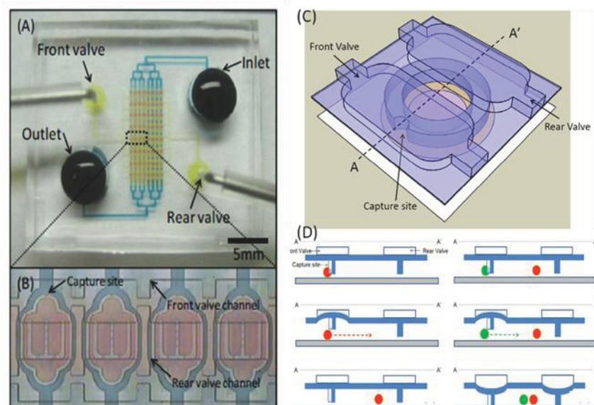
Figure 1: 1A) Device overview with connections, 1B) 2 Layer device with valve channel on top and capture site below, 1C) 3D device schematic, 1D) Principle of device operation
