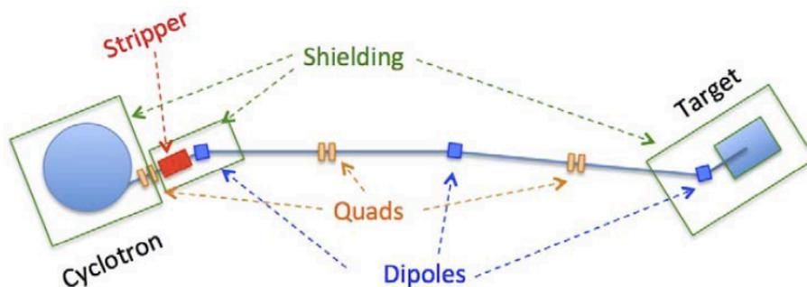
We must take the beam from the cyclotron to the target @ 60 MeV.
