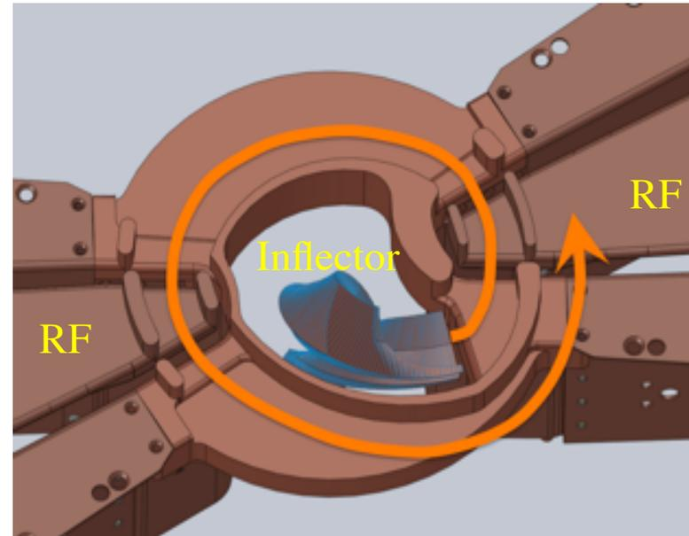
Most ions are lost in the first “turn” of the cyclotron because they hit material. (Phase acceptance 20-30 degrees)
