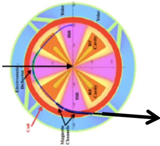
Avoid beam losses on the electrostatic extraction septum (protecting with a stripper foil, removing  $50 \mu\text{A}$  of beam)
