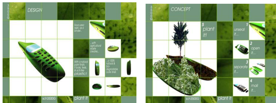
Figure 3. Sample eco-design of Cellular Telephone Housing (Parsons School of Design and University of Michigan). (Left) Bio-based soya resin concept for cell phone housing. (Right) Steps to recover cell phone circuit board and compost the bio-degradable housing lined with seeds.
