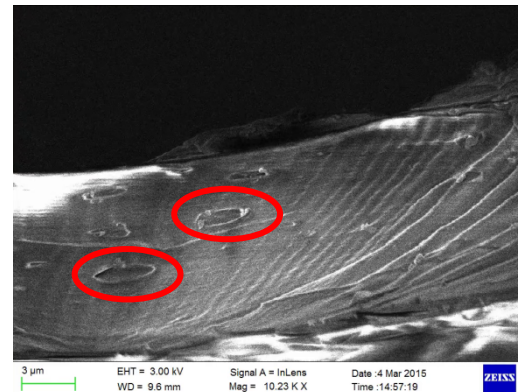
Scanning Electron Micrograph images of EPDM material near strained crack tip
