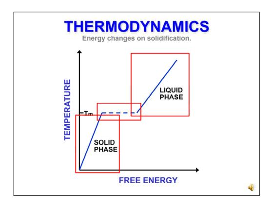
If you looked solely at the energetics of solidification, you would predict that everything occurred neatly at the freezing or melting temperature. We will use the abbreviation Tm to mean the temperature for melting or freezing. Tm implies that you are going up, but can also be used to talk about events when the temperature is going down.
