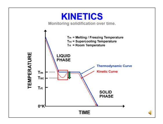
The blue curve that corresponds to the THERMODYNAMIC curve. Instead of T versus E, let's graph T versus t (time). **[CLICK]** What really happens on cooling is the red curve – which we call the KINETIC curve because it is related to time. On cooling from a high temperature, the cooling drops below the Tm, then recovers to the Tm, remains at Tm, and then begins to drop again. What is happening?
