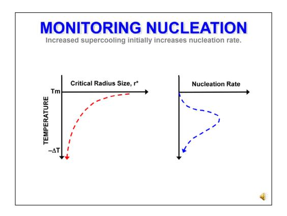
As shown in the previous slide, as the degree of supercooling increases, the critical radius size for a stable NUCLEUS gets smaller and smaller. That is why you do not tend to get supercooling below 20% of the absolute Tm. **[CLICK]** The odds of nucleation and grow rapidly increase with continuing supercooling but then falls off due to the decreasing thermal energy to get atoms to move around.
