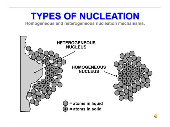
What we have described thus far is called HOMOGENEOUS NUCLEATION. It occurs within the liquid. Additionally, nuclei may also form at boundaries of the container for any liquid or at the surfaces of contaminants suspended in the liquid. These foreign surfaces are large enough to act as stable nuclei. These surfaces are called HETEROGENEOUS NUCLEI and material forming on these surfaces grows into normal grains. **[CLICK]**
