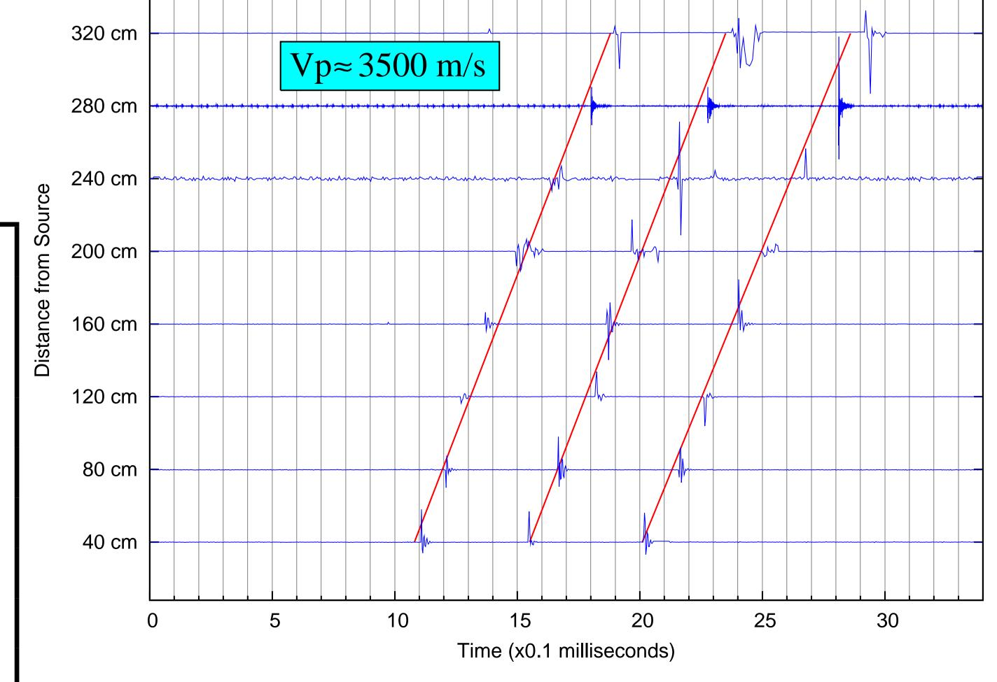
The compressed seismic section from the experiment. The red lines connect the first arrivals throughout the three shots.
