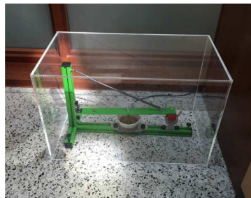
Figure 4: The exhibit seismometer at the F-Wing of Tech. This is a 1-component seismometer which only records vertical motions of the earth.
