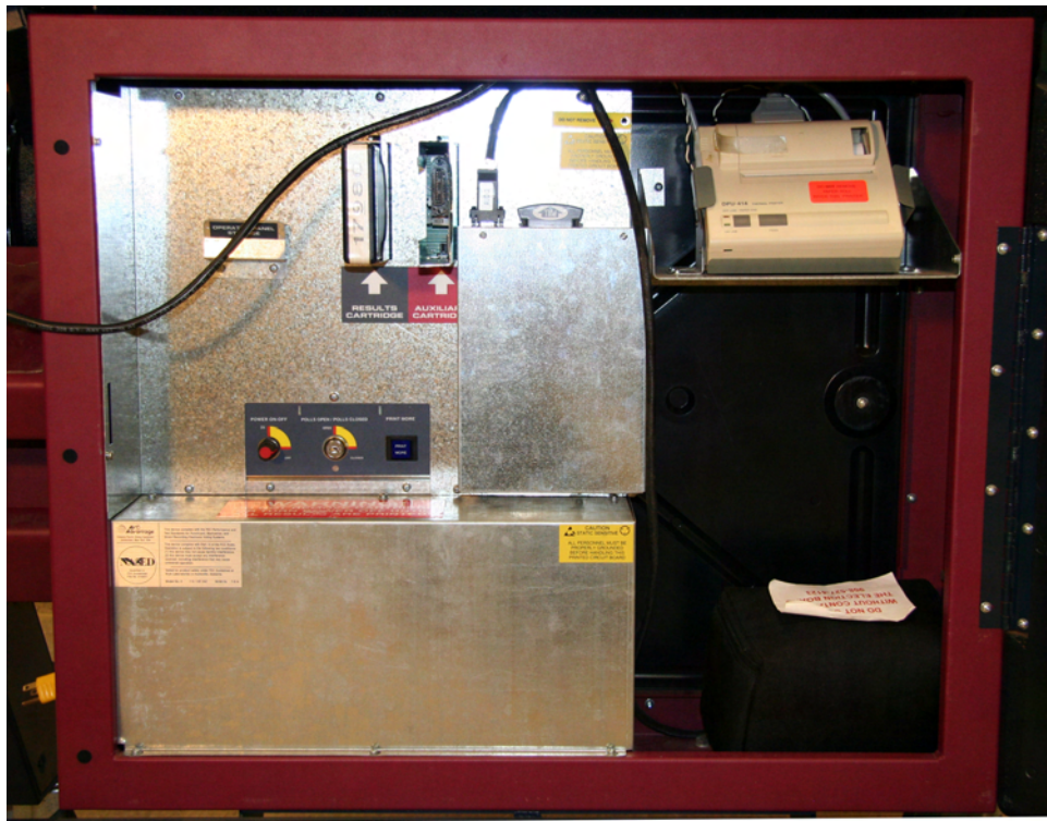
Figure 5: Inside the AVC Advantage cabinet, from the rear. Visible is the main circuit-board cover (sheet-metal, approximately 17x14 inches), through which protrude two ports, currently labeled “Results” and “Auxiliary.” In this picture, the Results port contains a Results Cartridge and the Auxiliary port is empty. To the right of these ports is a smaller metal box containing the audio-kit daughterboard, with a cable leading to a black nylon bag (at lower right) containing more audio-voting accessories. At center left are the power on-off knob, the polls open/closed keyswitch, and the “Print More” button. At upper right is a printer used for printing results reports. This machine is owned by Union County, NJ.
