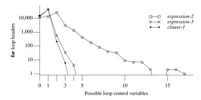
**Figure 1760.1:** Number of possible loop control variables appearing in *expression-2* (square-box) after filtering against the objects in *expression-3* (cross) and after filtering against the objects in *clause-1* (bullet). Based on the visible form of the .c files.
