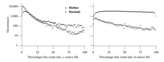
Figure 1838.2: Relative location (i.e., 100\*line\_number/lines\_in\_file) of #include and #define directives in the visible source.
