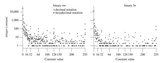
Figure 1202.2: Number of integer constants appearing as the right operand of equality operators. Based on the visible form of the .c files.
