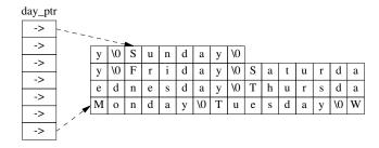
**Figure 986.2:** Difference in storage layout between an array of array of characters (left) and array of pointer to characters (right; not all pointers shown and the relative storage locations of the strings is only one of many that are possible).
