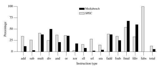
Figure 0.3: Percentage of *trivial* computations during program execution of the SPEC and MediaBench benchmarks for various kinds of operation. Adapted from Yi and Lilja.<sup>[1423]</sup>
