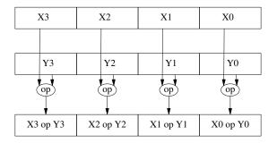
Figure 1368.1: Behavior of packed single-precision floating-point operations supported by the Intel Pentium processor. [607]
