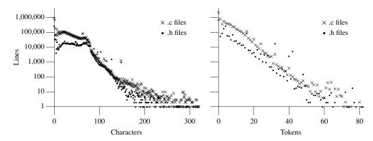
Figure 766.17: Number of non-white-space characters and tokens on a physical line; based on the visible form of the .c and .h files.
