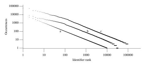
**Figure 787.26:** Identifier rank (based on frequency of occurrence of identifiers having a particular spelling) plotted against the number of occurrences of the identifier in the visible source of (b) Mozilla, and (c) Linux 2.4 kernel; (a) is a distribution following Zipf's law with the most common item occurring 10,000 times. Every identifier is represented by a dot.
