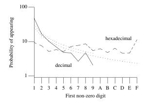
Figure 820.2: Probability of a decimal-constant or hexadecimal-constant starting with a particular digit; based on .c files. Dotted lines are the probabilities predicted by Benford's law (for values expressed in base 10 and base 16)—  $\log(1+d^{-1})$ , where d is the numeric value of the digit.
