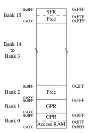
**Figure 555.1:** Data storage organization for the PIC18CXX2 devices<sup>[895]</sup> The 4,096 bytes of storage can be treated as a linear array or as 16 banks of 256 bytes (different instructions and performance penalties are involved). Some storage locations hold Special Function Registers (SFR) or General Purpose Registers (GPR). *Free* denotes storage that does not have a preassigned usage and is available for general program use.
