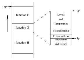
Figure 992.1: Common storage organization of a function call stack.
