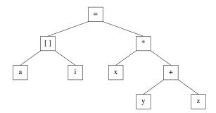
Figure 937.1: A simplified form of the kind of tree structure that is likely to be built by a translator for the expression a[i]=x\*(y+z).
