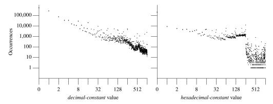
**Figure 820.1:** Number of integer constants having the lexical form of a *decimal-constant* (the literal 0 is also included in this set) and *hexadecimal-constant*, with different values. Based on the visible form of the .c and .h files.
