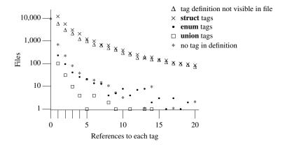
**Figure 1462.1:** Number of references to each tag previously defined in the visible source (times, bullet, square; the definition itself is not included in the count), tags with no definition visible in the .c file (triangle; i.e., it is defined in a header) and anonymous structure/union/enumeration definitions (star). Based on the visible form of the .c files.
