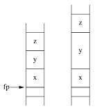
**Figure 1003.1:** An example of the impact, on relative stack addresses, of passing an argument having a type that occupies more storage than the declared parameter type. For instance, the offset of z, relative to the frame pointer, *fp* might be changed by passing an argument having a type different from the declared type of the parameter y (when there is no visible prototype, at the point of call, to cause the type of the argument to be converted).
