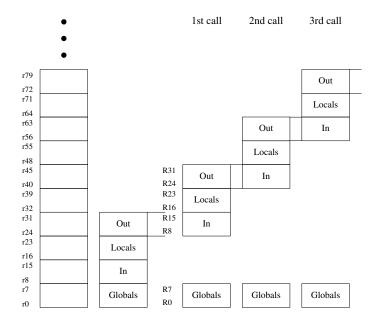
**Figure 996.1:** A processors register file (on the left) and the register windows, of registers accessible to a program, after 0, 1, 2, and 3 *call* instructions have been executed. The mapping of the first eight registers is not affected by the *call* instruction.
