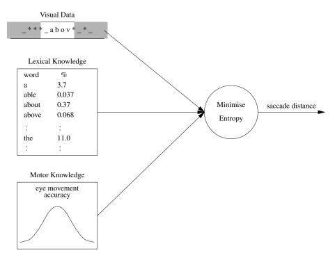
**Figure 766.12:** Mr. Chips schematic based on.<sup>[798]</sup> The shaded region in the visual data is the parafoveal; in this region individual letters (indicated by stars) can only be distinguished from spaces (indicated by underscores).
