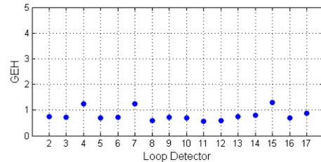
Fig. 6. Average GEH at each loop detector location
