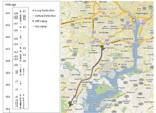
Fig. 1. Map for I-95 and the illustration of ramp and loop detector locations
