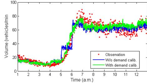
Fig. 2. Before and after the modification of OD demand matrix distribution during 5-7 am at loop detector #6
