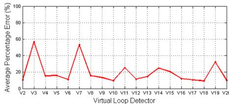
Fig. 8. Prediction error for the virtual detector locations
