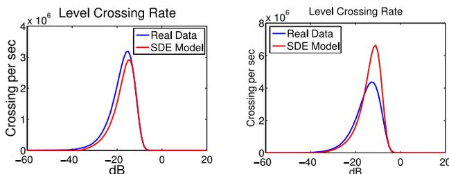
Fig. 6. Level crossing rate of synthesized SDE and measurement data (551 MHz left, 629 MHz right).
