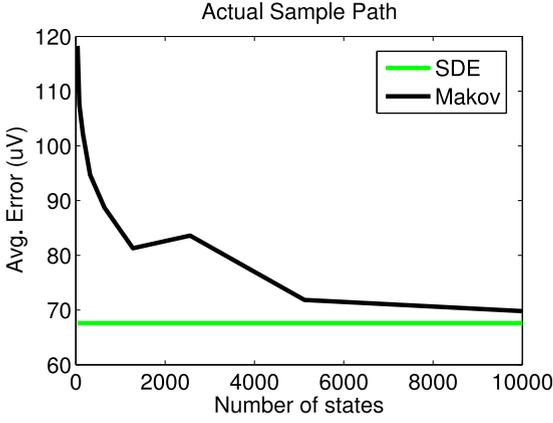
Fig. 12. Average error obtained using Markov models of different number of states compared with SDE.
