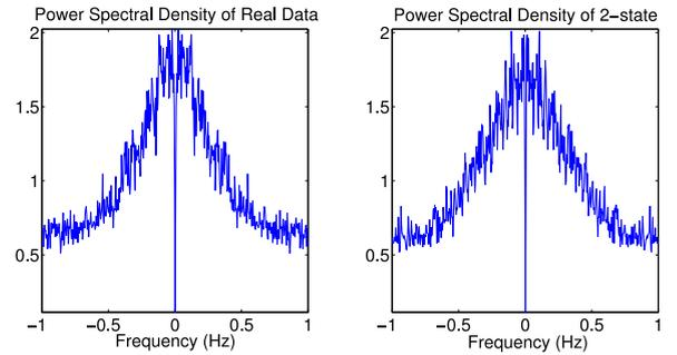
Fig. 10. The power spectral density of real data and the GE model over a 300-second duration.
