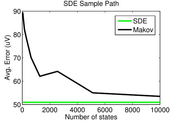
Fig. 13. Average error obtained using Markov models of different number of states compared with SDE.
