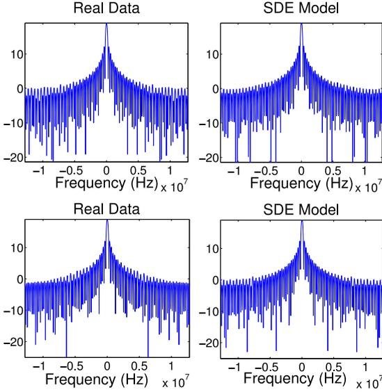
Fig. 5. Power spectral density of synthesized SDE and measurement data (551 MHz top, 629 MHz bottom).
