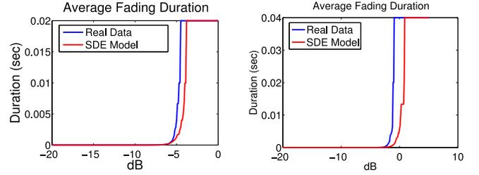
Fig. 7. Average fading duration of synthesized SDE and measurement data (551 MHz left, 629 MHz right).
