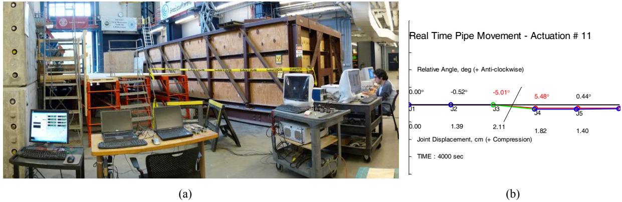
Fig. 8. Experimental setup: (a) data acquisition systems near the north test basin; (b) real-time pipeline movement after the 11 th actuation step.
