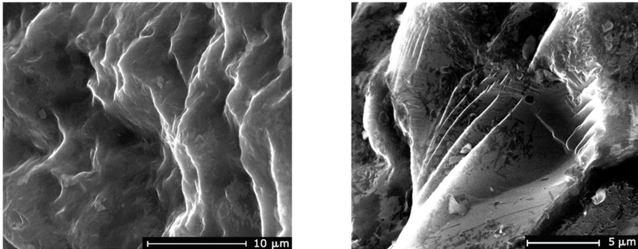
Figure 2. Morphology of sand grain surface: Ottawa 20-30 sand.
