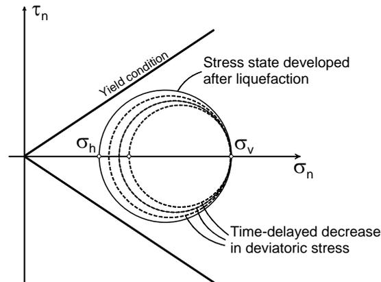
**Figure 4. Time-delayed reduction in deviatoric stress.**
