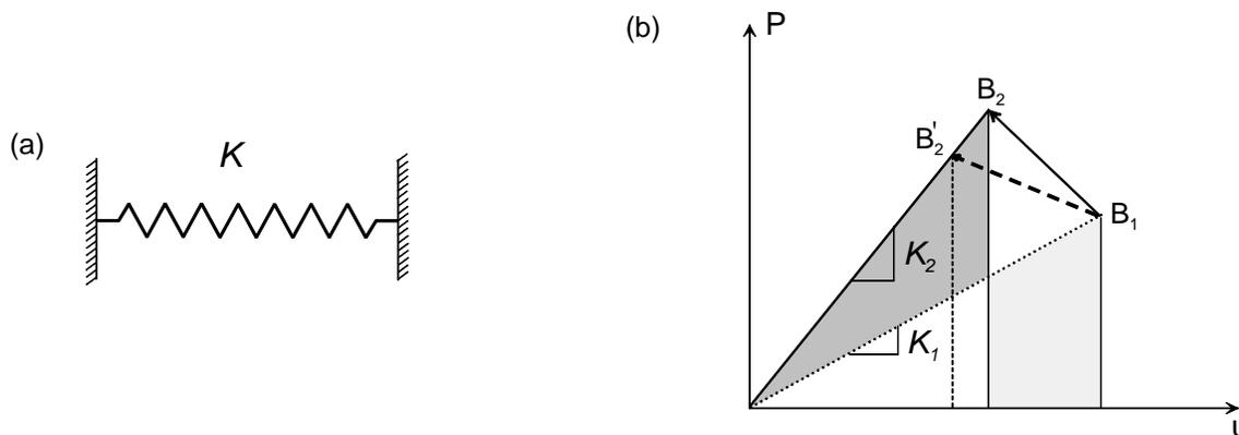
**Figure 3. (a) Spring between unyielding walls, and (b) balance of energy associated with an increase in the spring constant.**
