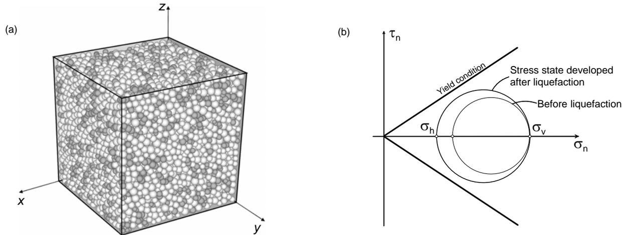
**Figure 1. (a) Discrete element model of a granular assembly, and (b) stress state before and after liquefaction (DEM simulation using  $PFC^{3D}$  code).**
