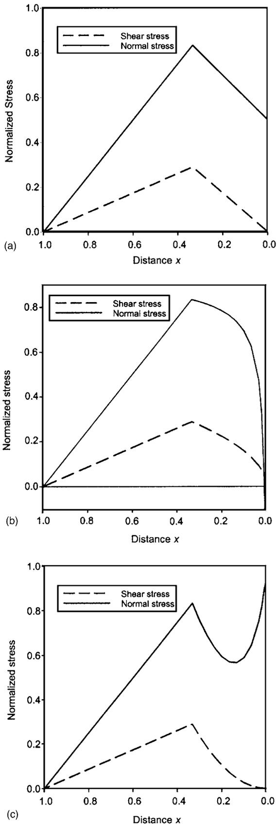
**Fig. 2.** Distribution of the contact stress at the base of a sand prism for different assumptions of  $\tau_{xy}$  in region  $OBC$ : (a) linear distribution; (b) square-root distribution; and (c) Jaky's parabolic distribution
