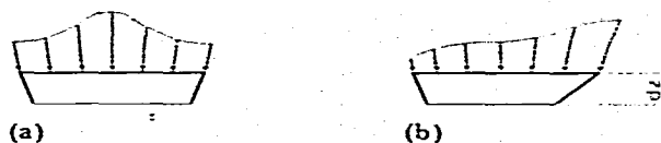
Fig. 1. Symmetrical slice with symmetrically distributed stresses (a), and asymmetrical slice (b).
