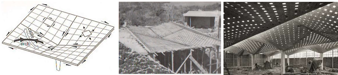
Figure 2: The straight line generators (left); steel reinforcement in Candela's typical shells (middle); 45° rotation of openings from edge in the High Life Textile Factory (right) [2]
