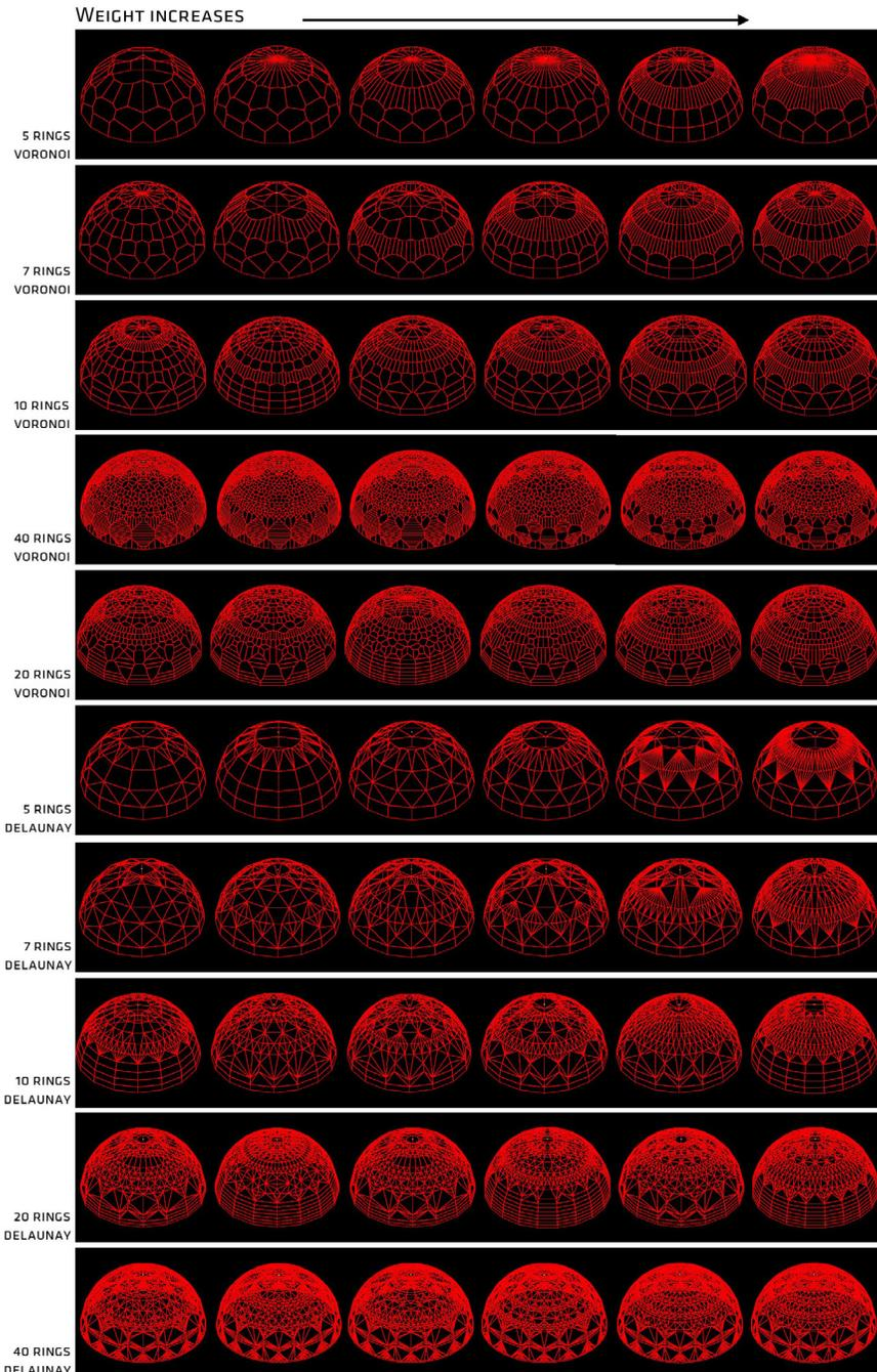
5. Selection of generated domes. Sorted by ring density and successively by weight of the structure.
