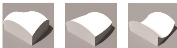
Figure 7: different shell curvatures affect the surface area of the surrounding walls, thus the walls are modeled adiabatic
