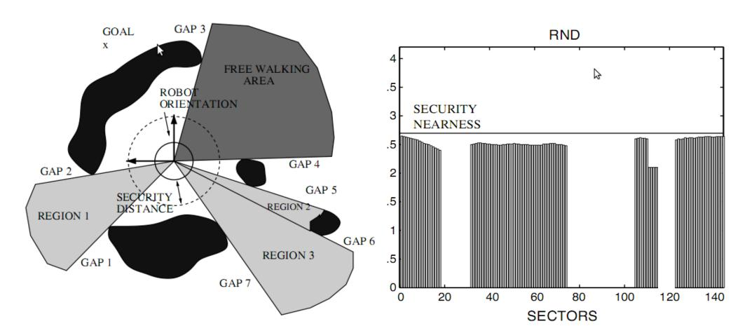
The first step is to define a distance beyond which an obstacle is not considered to be dangerous. Using the RND we find if any obstacles are there inside this security distance. If yes the situation is called Low Safety (LS), and if no obstacles are there in the security distance the condition is High Safety (HS). Next we divide the situation into 5 step.
