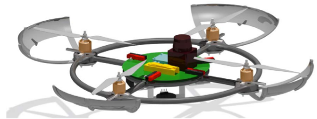
Figure 2: Image of MAAV's quadrotor design. From [1].
