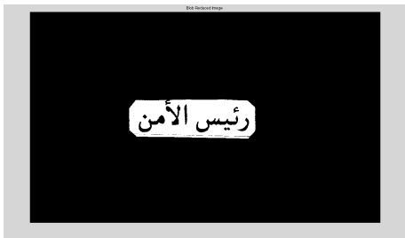
Figure 11: Segmentation of compound security sign post noise reduction by returning maximum white blob.
