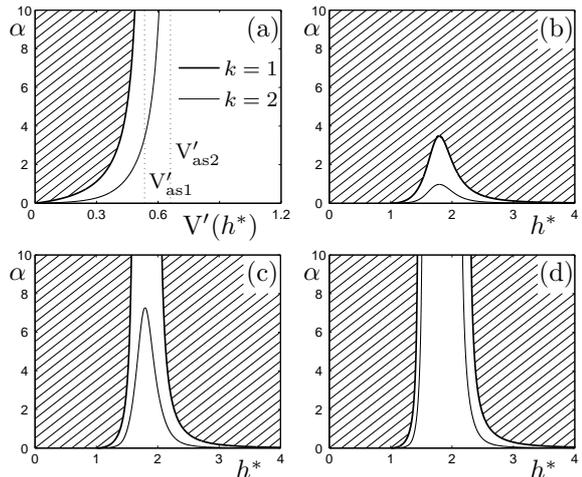
Fig. 2. Stability charts of the five-car system where shading denotes the stable region. Panel (a) shows the sensitivity  $\alpha$  as a function of the slope of the OV function  $V'(h^*)$ . Panels (b)–(d) show stability diagrams in the  $(h^*, \alpha)$ -plane, namely panel (b) for  $v^0 = 0.5$ , panel (c) for  $v^0 = 0.7$ , and panel (d) for  $v^0 = 1.0$ .
