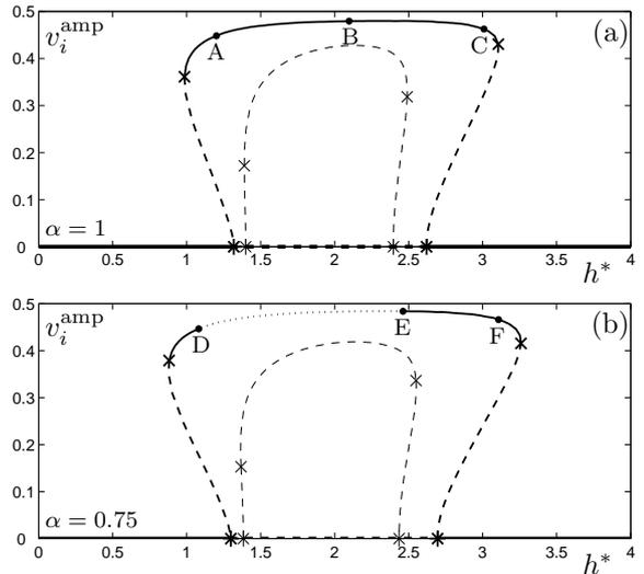
Fig. 4. Amplitude of oscillations of the velocity of the  $i$ -th car vs. average headway  $h^*$ . The horizontal axis represents the equilibrium state. Solid curves denote stable and dashed curves denote unstable states; the dotted curve represents the collision region. The bold and thin curves belong to the cases  $k = 1$  and  $k = 2$ , respectively. The value of  $\alpha$  is depicted in each panel and  $v^0 = 1$  for both (a) and (b).
