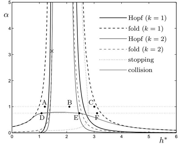
Fig. 3. Two-dimensional bifurcation diagram. The horizontal dotted lines correspond to the values of  $\alpha$  used in Fig. 4 and the marked points A–F correspond to the respective time profiles in Fig. 5
