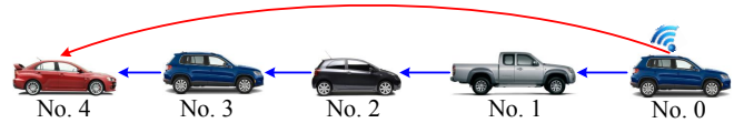
Fig. 3. A vehicle network where vehicle 4 monitors vehicle 3 and vehicle 0 while other vehicles only responds to the motion of the vehicle immediately ahead.
