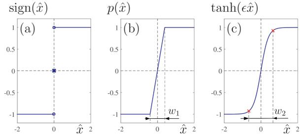
Fig. 2. (a): The non-continuous sign function (33). (b): The non-smooth piecewise linear function (34) with the width of boundary layer  $w_1 = 2\epsilon$ . (c): The infinitely smooth hyperbolic tangent function (35) with the width of boundary layer  $w_2 = \epsilon \ln(2 + \sqrt{3})$ . We set  $\epsilon = 0.4$  in (b,c).
