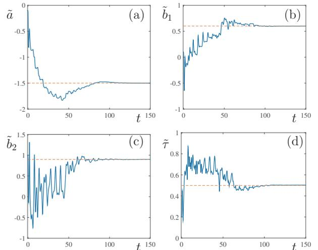
Fig. 4. Estimated feedback gains and delay time using the estimator (17). The dashed lines mark the real parameter values. The signals are generated using (4,5) with  $u_2(t) = \delta v_{i+1}(t) = \frac{2}{3}(\cos(t) + \cos(2.1t) + \cos(7t))$ . The estimator gains are  $\gamma_1 = 1.5$ ,  $\gamma_2 = 1.5$ ,  $\gamma_3 = 6.0$ ,  $\gamma_4 = 1.0$ .
