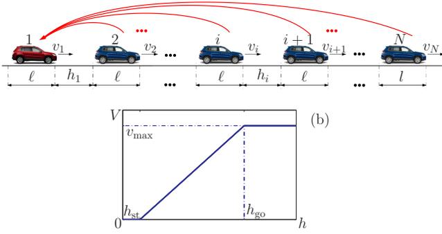
Fig. 1. (a): A string of  $N$  vehicles with a CCC vehicle at the tail receiving signals from human-driven vehicles ahead via wireless V2V communication. The red arrows denote information flow. The velocity of vehicle  $i$  is denoted by  $v_i$ . The bumper-to-bumper distance between vehicle  $i$  and vehicle  $i+1$  is called the headway and denoted as  $h_i$ . The length of every vehicle is assumed to be  $l$ . (b): The range policy function defined by (2).
