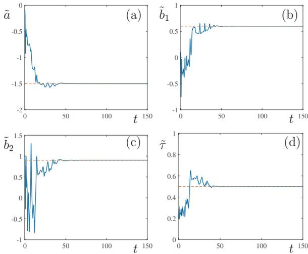
Fig. 5. Estimated feedback gains and delay time using the estimator (32,35). The notations and input signals are the same as in Fig. 4. The estimator gains are  $\gamma_1 = 1.5$ ,  $\gamma_2 = 1.5$ ,  $\gamma_3 = 4.0$ ,  $\gamma_4 = 0.35$ , and we set  $\epsilon = 0.4$ .
