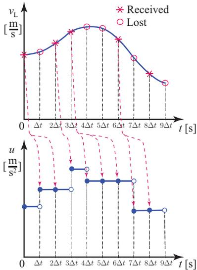
Fig. 2. Top: Sampling a continuous signal using wireless communication. Bottom: A zero-order-hold control signal based on the received packages.
