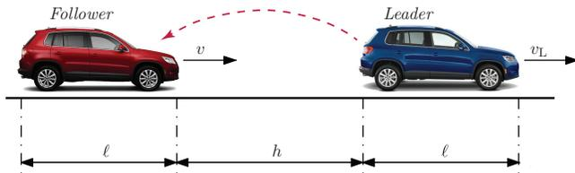
Fig. 1. Simple car-following configuration.
