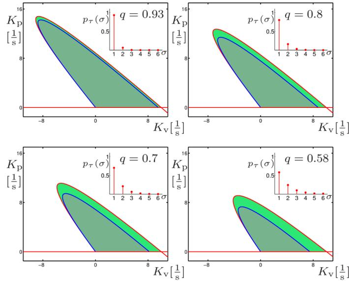
Fig. 3. Stability charts for different packet delivery ratios  $q$  as indicated (and shown by inlets). The outer curve envelops the mean stable region, while within the dark shaded domain point-wise asymptotic stability is achieved. The other parameters used here are  $v_{\max} = 30\text{m/s}$ ,  $h_{\text{st}} = 5\text{m}$ ,  $h_{\text{go}} = 35\text{m}$ ,  $v^* = 15\text{m/s}$ ,  $\Delta t = 0.1\text{s}$ ; cf. equation (39).
