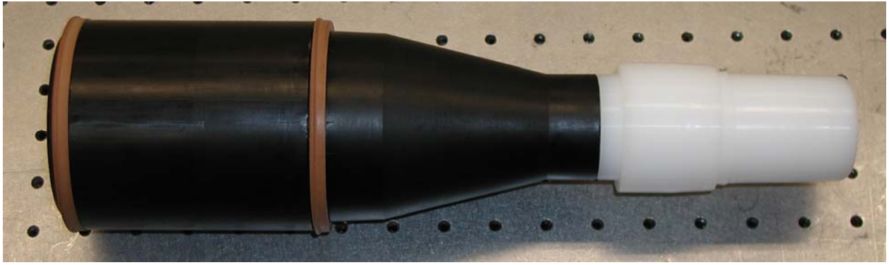
Fig. 4 Photograph of the UM-RCF sabot. The black portion is the Delrin™ body and the white portion is the UHMW replaceable nose cone. The two U-ring seals can be seen on Delrin™ section of the sabot.
