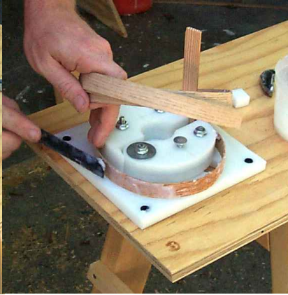
13) Apply epoxy to the outside of the strip, lay it in place and pull tightly as you go around.
