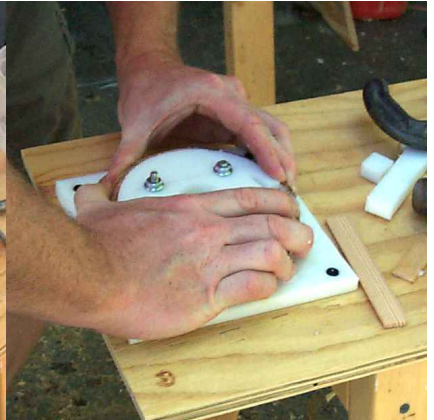
17) Remove the wedge. Holding the hoop in place, remove the clamp. Twist the entire hoop clockwise to free the starting end of the hoop.
