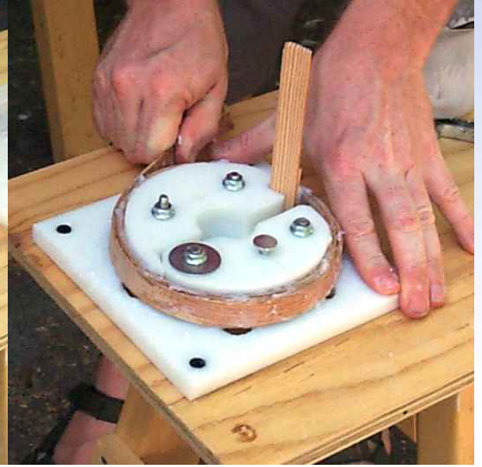
14) When the entire strip is glued, pull on the free end to take out any remaining slack.
