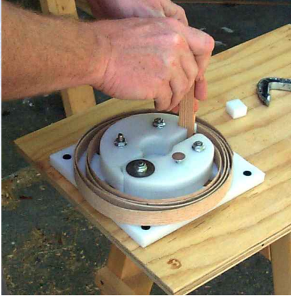
12) Secure the inner end of the hoop in the slot with a small wedge.
