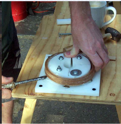
22) If necessary, pry the hoop upwards with a screwdriver in the knockout holes.
