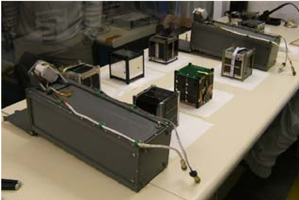
Figure 1: Six CubeSats and their deployment systems.
