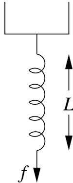
has a spring constant and resting length that depend on temperature, so that we need to use thermodynamics to calculate its behavior.
