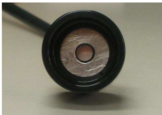
Figure 3.1: Picture of a piece of the spot-o-matic tube. In the center of the tube is a faint, small red dot. This red dot is light emerging from the 10 micron pinhole after having passed through the fiber optic and through a 650 nm narrow bandpass filter. This red dot is what is imaged by the lens system of the spot-o-matic and onto the FPA.
