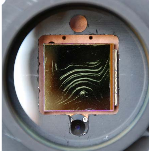
Figure 1.1: Picture of H2-103, one of the NIR detectors that have been tested in the SNAP laboratory.
