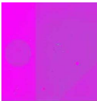
Figure 3.1: Image of a Flexible Image Transport System (FITS) file. FITS is used to store and process images in a digital file format. In the SNAP laboratory FITS files are supported by SAO Image DS9. The FITS image above was taken by H2-103 at peak wavelength 1300 nm. A FITS file represents an array of every pixel value in the detector.
