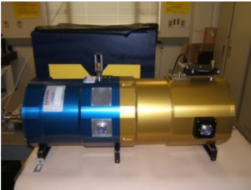
Figure 2.2: Existing DEWAR (blue) mated with new extension (gold). Light source and introductory optics not pictured.
