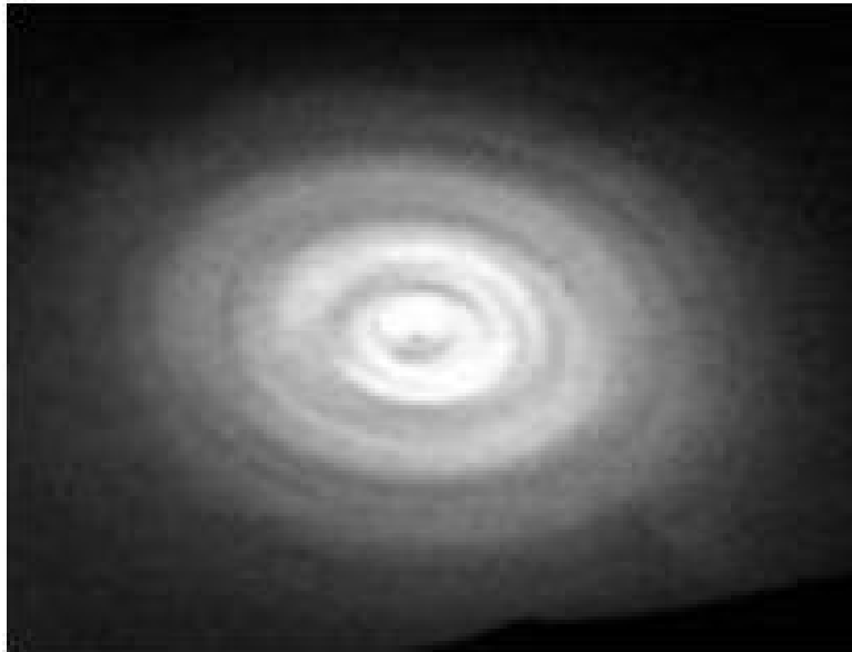
Figure 2.7: The pattern emitted by the glass rod before the introduction of the diffusion paper.
