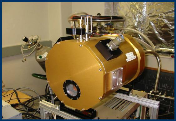
Devices are mounted in a dewar and kept at 140K to reduce dark current and simulate deep space conditions
