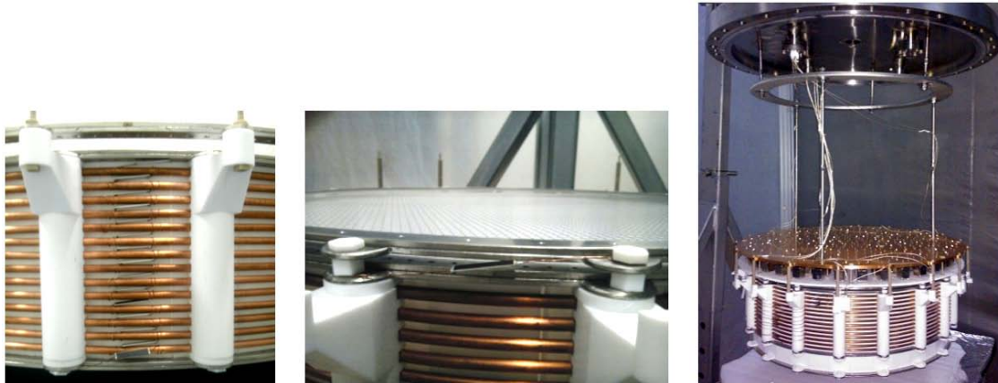
Figure 5.7.1: Left: Photograph of the resistor chain attached to the field shaping rings. The resistors linearly drop voltage vertically across the drift volume. Center: Photograph of the anode and gate electrodes. Right: Assembled TPC before the Run5. Figure from [84].
