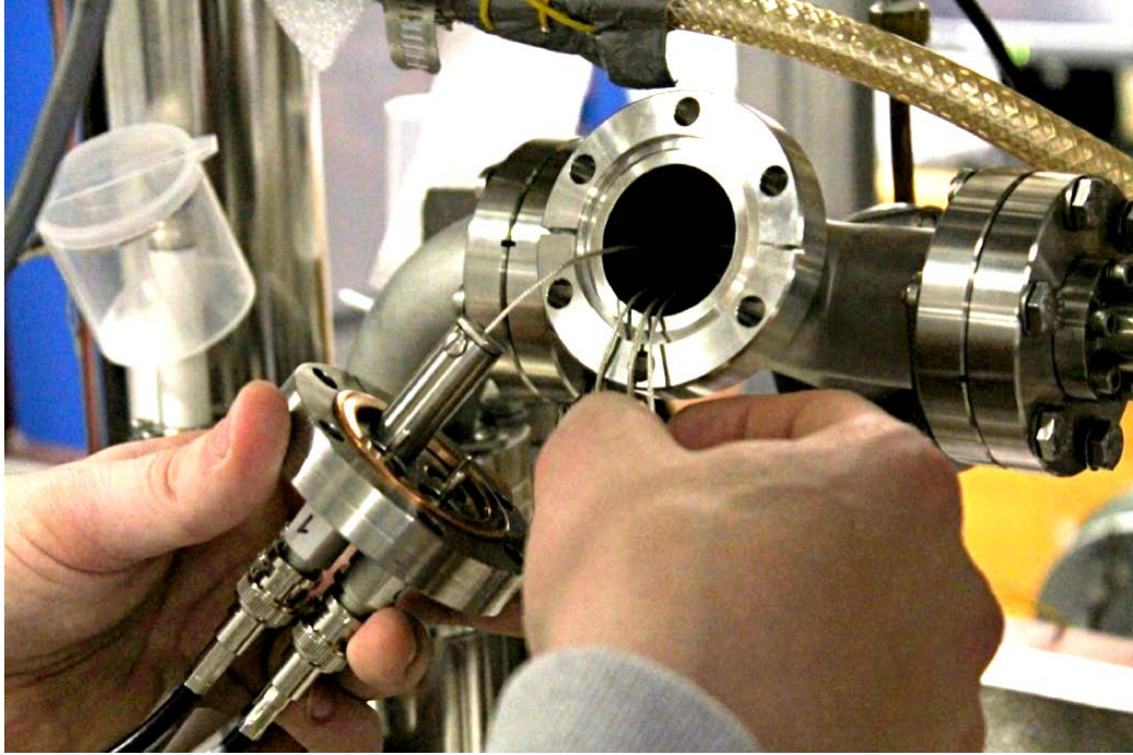
Figure 4.1.5: A photograph of the custom SHV-BNC feedthrough connectors and cabling used in MiX. Standard vacuum BNC connectors breakdown readily in gaseous xenon above O(1 \text{ kV}) . The connectors and cabling were produced in-house to allow for transport of the high voltages necessary for the PMTs. Connector design courtesy of Curtis Weaverdyck.
