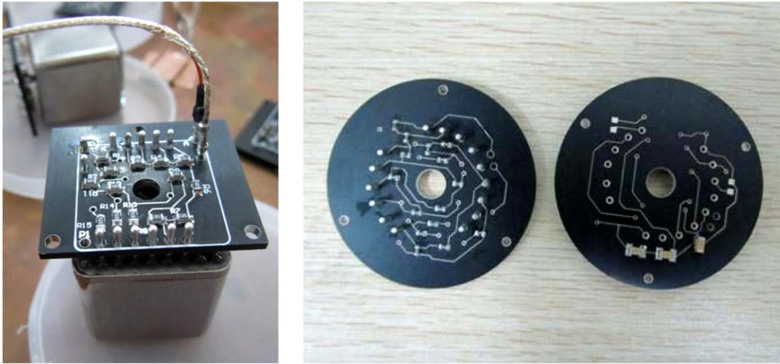
Figure 5.6.6: Left: Photograph of the Cirlex base for the top PMT attached to a Hamamatsu R8520-406. Right: Photograph of both sides of the Cirlex bottom PMT base. In both top and bottom cases, the Cirlex with deposited silver traces provides a very low outgassing substrate, reducing the offgas load in the inner vessel. Figure from [84].
