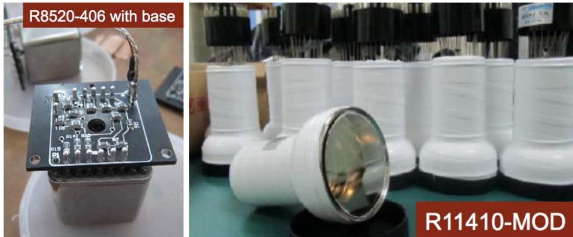
Figure 5.6.4: Left: Photograph of a top PMT is shown after assembly and testing with attached voltage dividing base circuit and cable assembly. Right: Photograph of a collection of bottom PMTs during characterization. The external teflon wrap is for protection during handling and is removed before insertion in the TPC.
