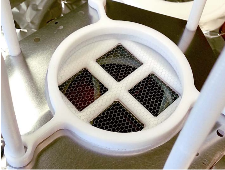
Figure 4.1.6: A photograph of the chemically etched mesh used for all electrodes in the MiX TPC (anode shown). The 50\ \mu\text{m} -thick mesh has a central 76 mm circular region with hexagonally packed grid structure. The hexagons are created at a 2 mm pitch with 50\ \mu\text{m} diameter wires to allow for homogenous TPC field generation while maintaining 95% optical transparency.
