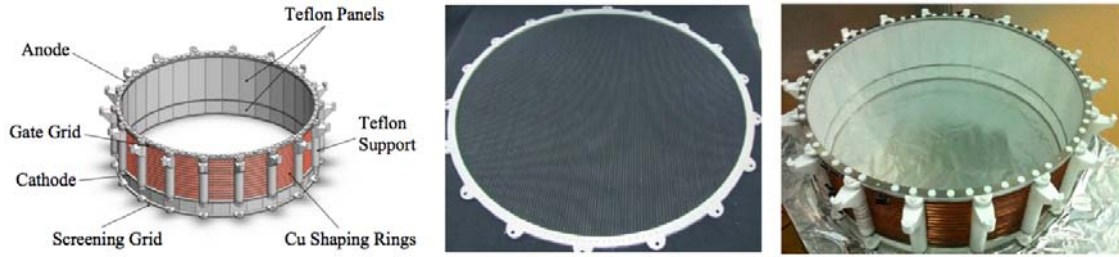
Figure 5.6.3: Left: Schematic of field shaping cage and electrodes. A grounded anode caps the top of the high electric field region, the gate voltage sets the extraction field, and the cathode voltage sets the drift field. A set of 14 field shaping rings sets the voltage boundary conditions to maintain a uniform field in the TPC. Center: Photograph of a gate, cathode, and screening electrode unit formed of parallel 200\ \mu\text{m} wires at 5\ \text{mm} pitch. Right: Photograph of assembled electrodes and field cage with cylindrical reflector. Figure from [84].
