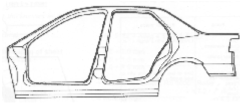
Figure 4. A side frame of a passenger car used in case studies.
