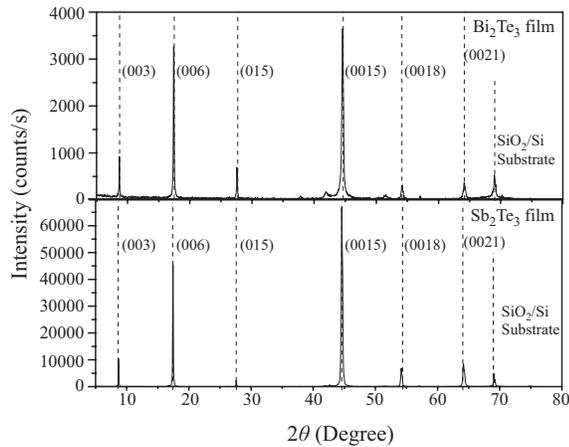
FIG. 6. X-ray diffraction spectrum for optimal  $\text{Bi}_2\text{Te}_3$  and  $\text{Sb}_2\text{Te}_3$  films.
