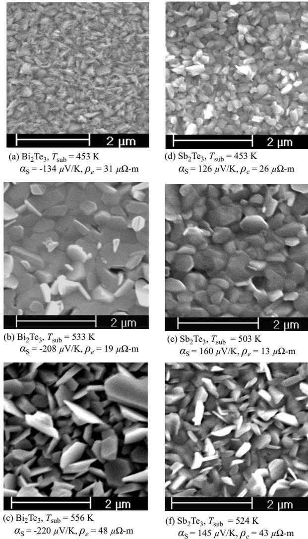
FIG. 4. [(a)–(c)] SEM micrographs of the  $\text{Bi}_2\text{Te}_3$  films deposited at different substrate temperatures with a FR of 2.4. [(d)–(f)] SEM micrographs of the  $\text{Sb}_2\text{Te}_3$  films deposited at different substrate temperatures with a FR of 3.0.
