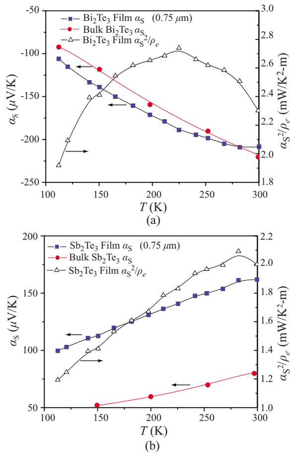
FIG. 9. (Color online) Temperature dependence of the Seebeck coefficient and power factor of the deposited (a) Bi<sub>2</sub>Te<sub>3</sub> and (b) Sb<sub>2</sub>Te<sub>3</sub> films. The Seebeck coefficients of bulk Bi<sub>2</sub>Te<sub>3</sub> and Sb<sub>2</sub>Te<sub>3</sub> films reported in the literature (Refs. 9 and 19) are also shown.
