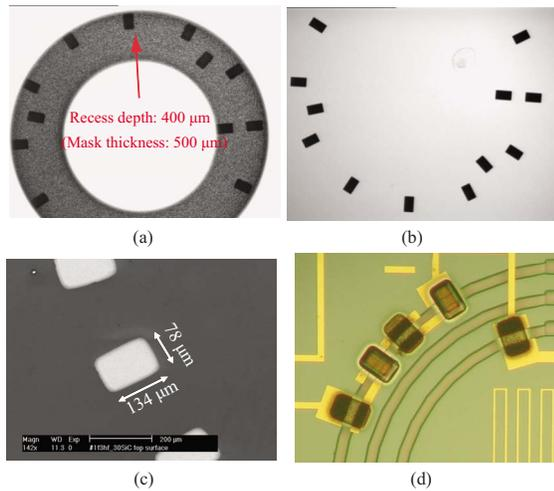
FIG. 10. (Color online) (a) Top view of the fabricated Si shadow mask. (b) Bottom view of the fabricated Si shadow mask. (c) Deposited  $\text{Bi}_2\text{Te}_3$  patterns using the shadow mask. (d) Aligned  $\text{Bi}_2\text{Te}_3$  and  $\text{Sb}_2\text{Te}_3$  film patterns.
