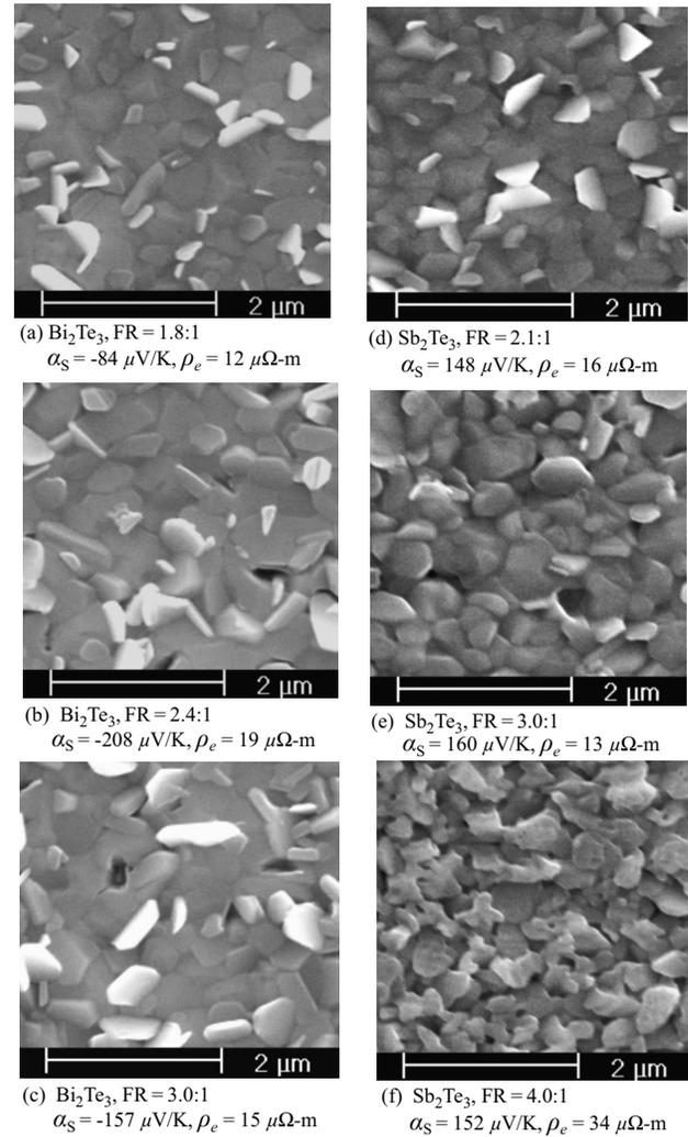
FIG. 5. [(a)–(c)] SEM micrographs of the  $\text{Bi}_2\text{Te}_3$  films deposited with different evaporation FRs at 533 K. [(d)–(f)] SEM micrographs of the  $\text{Sb}_2\text{Te}_3$  films deposited with different evaporation FRs at 503 K.
