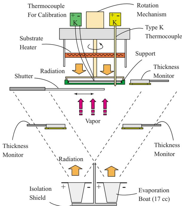
FIG. 1. (Color online) Schematic of coevaporation system.
