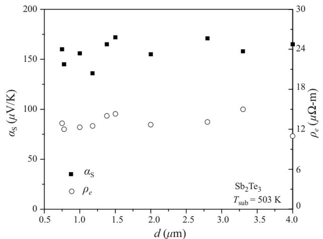
FIG. 2. Variation in Seebeck coefficient and electrical conductivity of Sb<sub>2</sub>Te<sub>3</sub> films (deposited with  $T_{\text{sub}}=503 \text{ K}$  and  $\text{FR}=3.0$ ) with respect to the film thickness.
