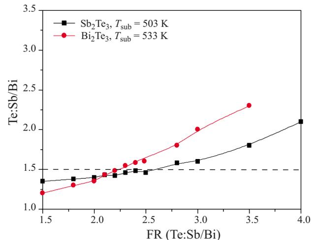
FIG. 3. (Color online) Variation in film composition ratio Te/Bi(Sb) with respect to FR at the optimal  $T_{\text{sub}}$ , i.e.,  $T_{\text{sub}}=533$  K for  $\text{Bi}_2\text{Te}_3$  and 503 K for  $\text{Sb}_2\text{Te}_3$ .
