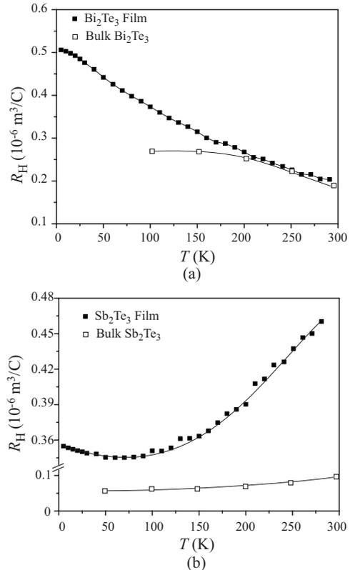
FIG. 7. Temperature dependence of the Hall coefficients of the optimal (a)  $\text{Bi}_2\text{Te}_3$  and (b)  $\text{Sb}_2\text{Te}_3$  films. The experimental results for bulk materials (Refs. 15 and 19) are also shown.
