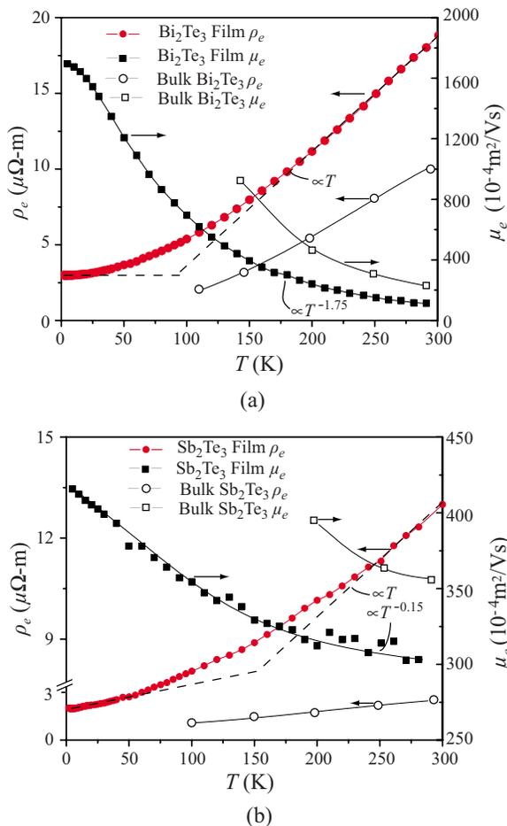
FIG. 8. (Color online) Temperature dependence of the electrical resistivity and the mobility of the deposited (a) Bi<sub>2</sub>Te<sub>3</sub> and (b) Sb<sub>2</sub>Te<sub>3</sub> films. The experimental results for bulk materials (Refs. 15 and 19) are also shown.
