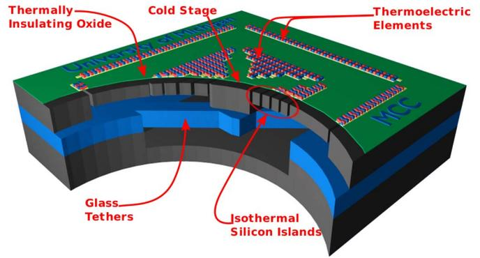
Fig. 1. Three-dimensional rendering of the six-stage TE microcooler showing its major components, including the isothermal silicon islands, insulating dielectric, supporting glass, and TE elements.
