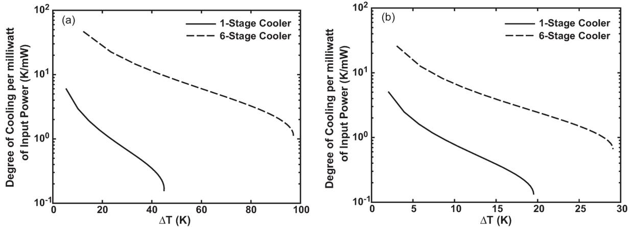
Fig. 6. (a) Predicted degree of cooling per milliwatt as function of cooling for ideal one- and six-stage coolers. (b) Predicted degree of cooling per milliwatt for one- and six-stage coolers, taking into consideration contact resistivity of  $1.24 \times 10^{-8} \Omega \cdot \text{m}^2$  and a  $1.5\text{-}\mu\text{m}$ -thick layer of oxide supporting the TE material.
