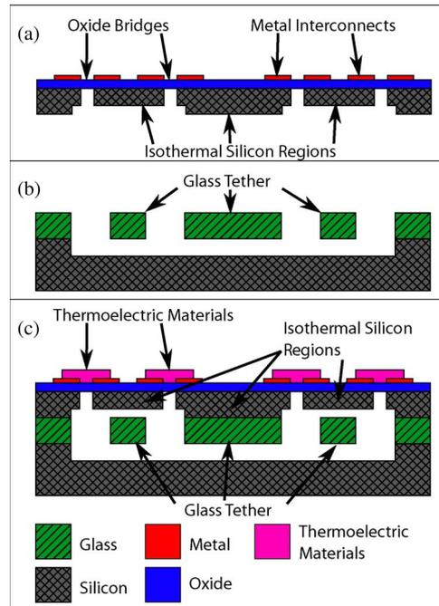
Fig. 2. (a) Cross-sectional view of the “thermal substrate” fabricated from a 100-μm-thick silicon wafer. (b) Cross-sectional view of (middle) “structural substrate,” which contains a suspended glass tether used to support the cold stage. (c) Cross-sectional view of the completed cooler.
