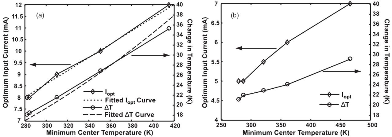
Fig. 8. (Left axes) Optimum input current and (right axes) change in temperature between the OFF and ON states at the center of the cooler under varying thermal load conditions. In all cases, the ambient temperature is maintained at 300 K, and the temperature of the center region is increased by applying a thermal load with a resistive element. (a) Results from a one-stage cooler, along with curves fitted to the physical model. (b) Results from a six-stage cooler.
