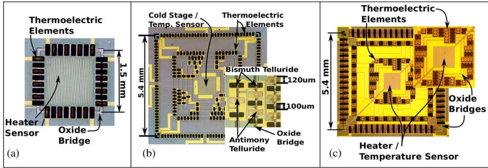
Fig. 3. Top-down micrographs of (a) a one-stage cooler, (b) the Version-1 six-stage cooler with visible cold stage, isothermal islands, and TE elements, and (c) the Version-2 six-stage cooler, with a different isothermal island spacing and a different TE element configuration from (b). The insets highlight the TE elements and oxide bridges.
