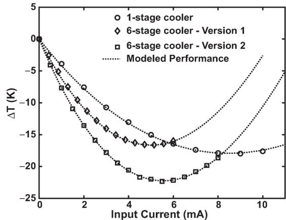
Fig. 7. (Symbols) Measured versus (lines) modeled performance of both versions of the six-stage cooler and the one-stage cooler. Material properties were used as simulation parameters to fit the model to the measured results.
