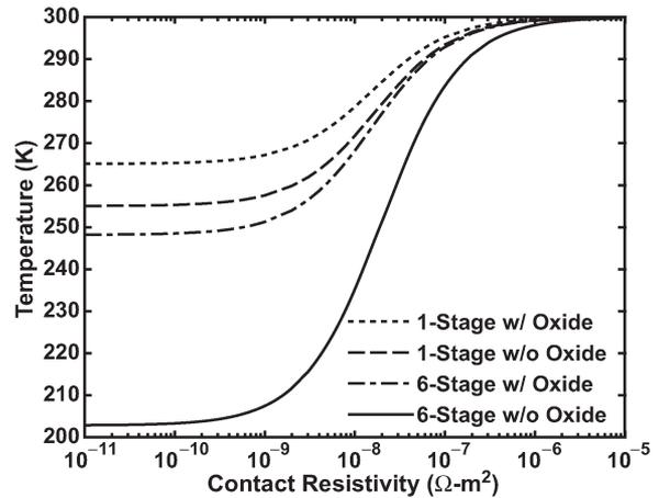
Fig. 5. Variation in thermal performance of one- and six-stage coolers simulated as a function of the contact resistivity. Both cooler designs are simulated under ideal conditions with no oxide supporting the TE material and under realistic conditions with 1.5  $\mu\text{m}$  of oxide. The TE material properties and geometric parameters used in the simulations can be found in Tables II and III.
