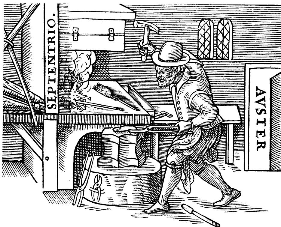
Figure 16.1: A woodcut from William Gilbert's treatise on magnetism (1600). It shows the manufacture of a magnetized bar. If the bar is heated and then placed on the anvil so that its ends are oriented towards magnetic north ( septentrio ) and south ( auster ), then after the bar cools, it is magnetized. This suggested to Gilbert (correctly!) that the earth itself was a magnet.
