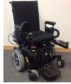
Fig. 6. The wheelchair robot (0.76 × 1.2 m). The wheelchair is differentially driven, such that linear and angular velocity are controlled independently. The robot is underactuated that the linear velocity is always aligned with the orientation of the robot (i.e. the robot cannot move sideways). The motor becomes saturated at linear and angular accelerations of 0.4 m/s 2 and 1.0 rad/s 2 . The robot model for the forward prediction fully reflects the constraints.
