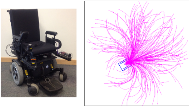
Fig. 2. Left: The wheelchair robot ( 0.76 \times 1.2\text{m} ). The wheelchair is differentially driven, such that linear and angular velocity are controlled independently. The robot is underactuated such that the linear velocity is always aligned with the orientation of the robot (i.e. the robot cannot move sideways). The motor becomes saturated at linear and angular accelerations of 0.4\text{m/s}^2 and 1.0\text{rad/s}^2 . The robot model for forward prediction fully reflects these constraints. Right: Randomly selected 300 samples from the continuous space of smooth and realizable closed-loop trajectories, parametrized by the four dimensional vector z_* = (r, \theta, \delta, v_{\max})^T over a time horizon [0, T] . The trajectories shown are generated from the dynamically simulated vehicle (with non-holonomic constraints and actuator saturations) under the stabilizing kinematic controller.
