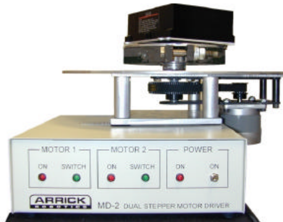
Figure 2: The KVH E-Core RD2100 mounted on the Arrick Robotics stepper motor-driven 4:1 reduction gear that served as a rotary table during experimentation.
