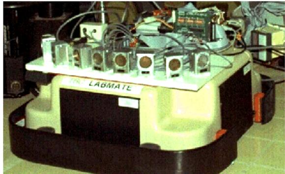
**Figure 7:** One of the four TRC LabMates at the University of Michigan. The system shown here is equipped with 8 ultrasonic sensors that were not used in the UMBmark experiment.
