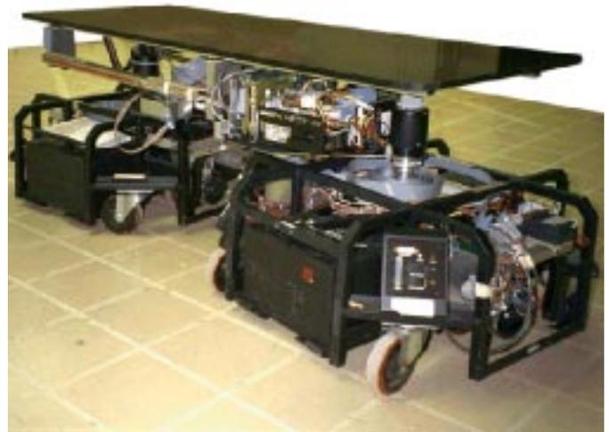
**Figure 8:** The CLAPPER is a unique 4-DOF mobile robot developed at the University of Michigan. The CLAPPER can measure and correct *non-systematic* odometry errors during motion.
