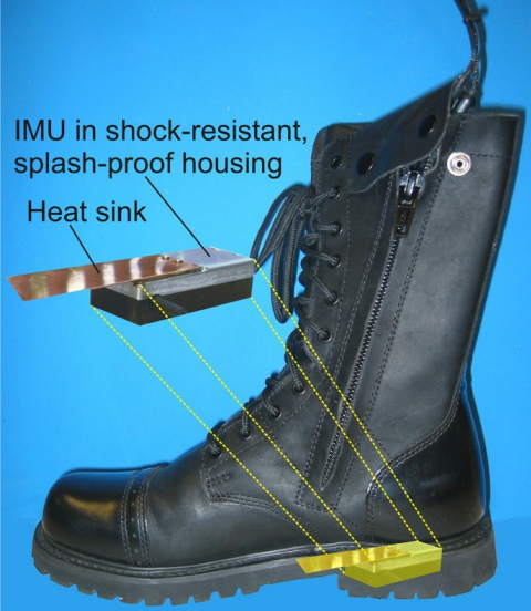
Figure 1: The PDR system uses an IMU mounted inside the heel of the user’s boot. Other mounting options exist but are not shown here.
