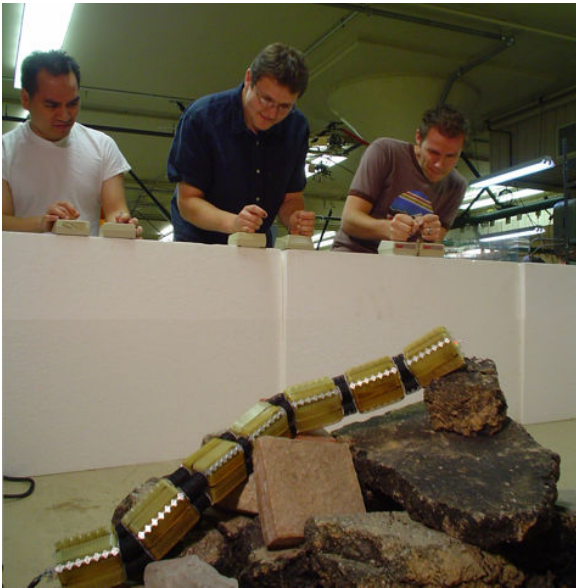
Figure 1: Three highly trained operators are currently needed in order to control the OT-4 with its 13 DOF.
