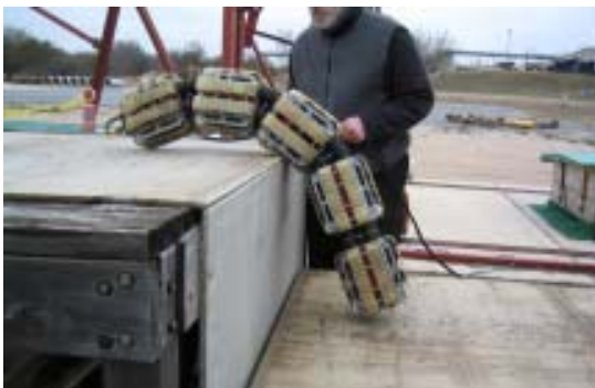
Figure 6: OmniTread climbing over an edge. At this moment almost all the weight of the robot rests on the tracks contacting the edge. Tracks of too elastic a material would slip out of the sprockets under such loads.
