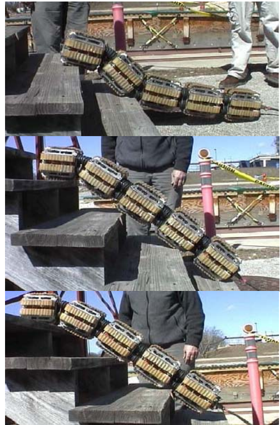
Figure 14: Sequence of photographs showing the OmniTread climbing up a flight of wooden stairs.
