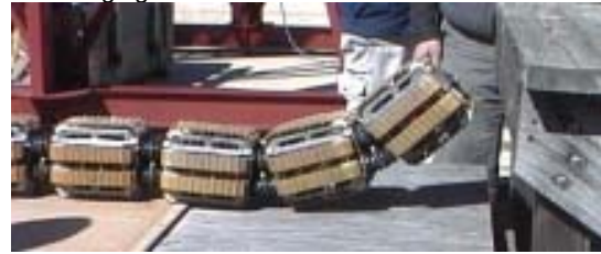
Figure 4: The OmniTread successfully crosses a gap that is a little wider than half the robot's length. By lifting its front segments up, the center of gravity shifts slightly toward the rear.
