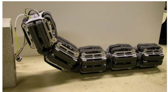
Figure 11: Experiments with OmniTread lifts up its two lead segments.
