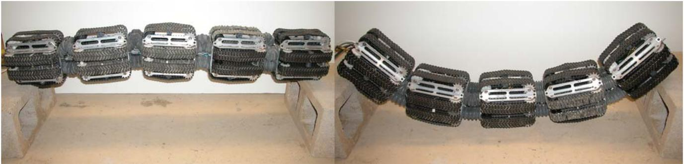
Figure 12: Experiments with active stiffness control. a) maximum stiffness – left, b) minimum stiffness – right.
