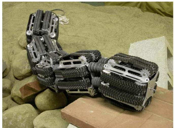
Figure 2: The OmniTread serpentine robot developed at our lab. As in the OmniPede, a single drive motor housed in the center segment powers a drive shaft spine, from which torque is derived for all treads. All segments are linked by 2-DOF pneumatically actuated joints, which are the focus of this paper.
