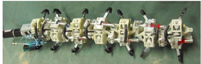
Figure 1: The “OmniPede,” developed at our lab, is a 7-segment serpentine robot that uses legs for propulsion. An electric motor at the end rotates a so-called “drive shaft spine,” which provides mechanical power to each foot (black parts) through a five-bar mechanism. Segments are linked by 2-DOF articulate joints that are actuated by two pneumatic cylinders.
