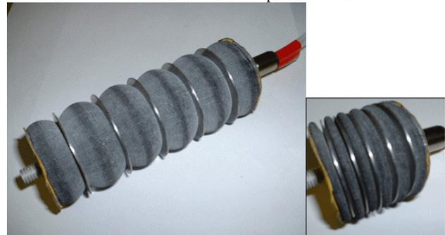
b. Pneumatic bellows, extended and compressed
